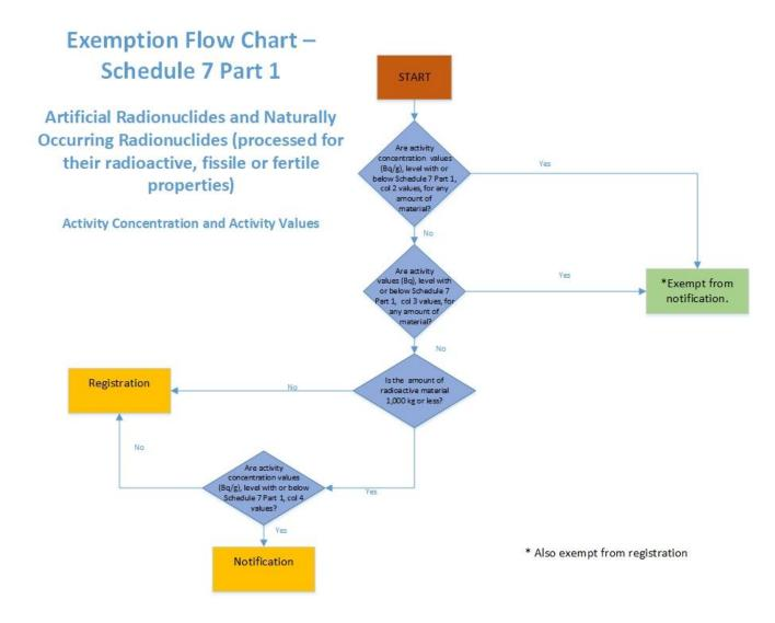
Flowchart showing which level of the graded approach applies for work with artificial radionuclides and naturally occurring radionuclides which are processed for their radioactive, fissile or fertile properties that require notification
